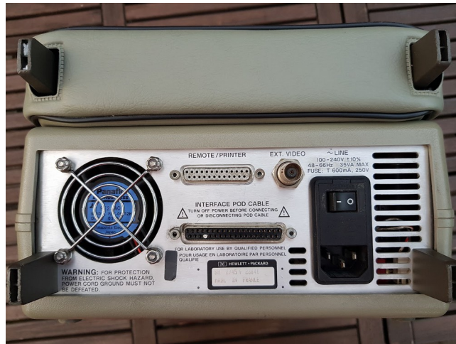
Figure 9: Rear view with combination of IEC plug, filter, fuse and switch
