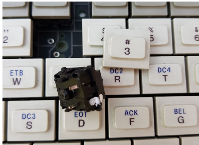
Figure 10: Desoldered key
