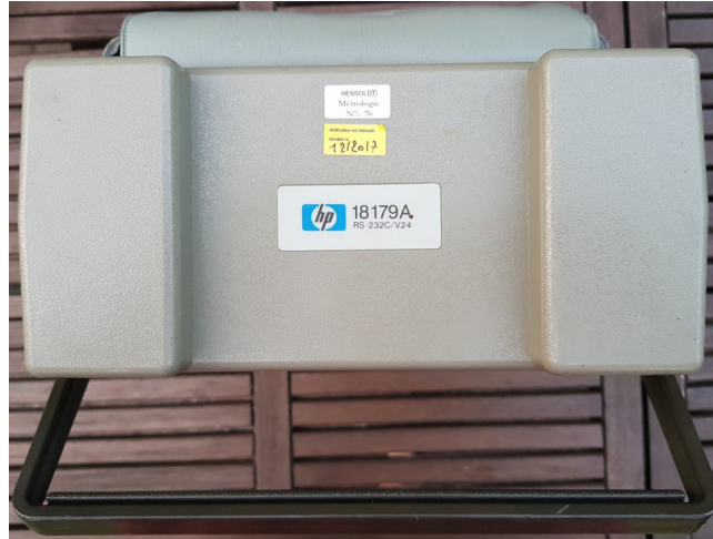
Figure 4: Front view with RS232C Interface Pod
